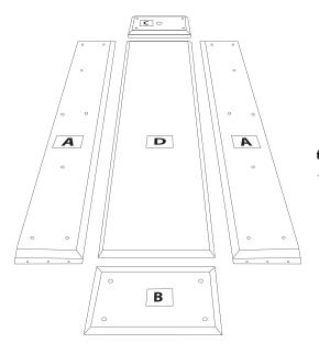
Assemble box side walls (parts A, A, B, C) using included 1 1/4" screws and pilot holes.
