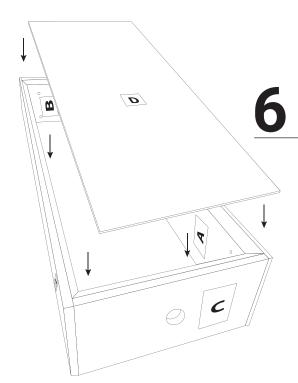
For 39" Drywall box: Place one L bracket on each corner.
